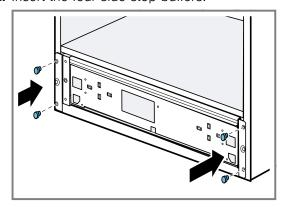
9. Remove the retaining plate from the appliance.
