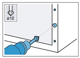
7. Drill the 4 holes for the stop buffers.
