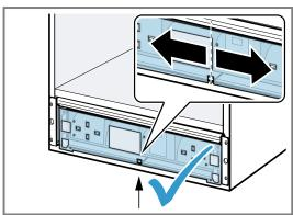
7. Screw the appliance into the fitted unit using the two long screws.
