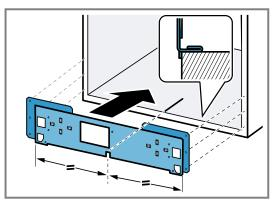
5. Mark the 6 holes on the front edge of the fitted unit.
