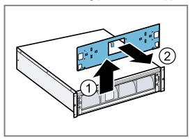
3. Attach the metal plates to the retaining plate on both sides.
