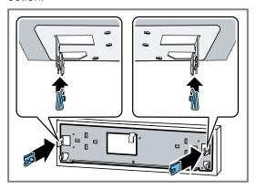
5. Attach the furniture panel to the appliance using the retaining plate.
