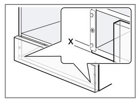
2. Position the retaining plate on the rear of the furniture panel and align it.
