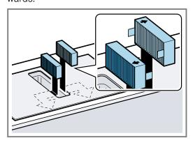
5. Insert the other odour filters or acoustics filters into the left and right of the appliance.
