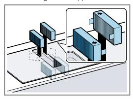
6. Insert the grease filter.
