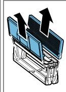
2. Place the individual components of the grease filter loosely in the dishwasher and do not jam them in.
