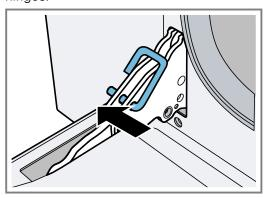
The locking pins must be fully inserted into the holes in the hinges.
