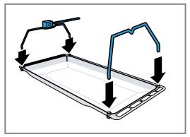
2. Place the rotary spit onto the rotary spit frame and unscrew the handle.
