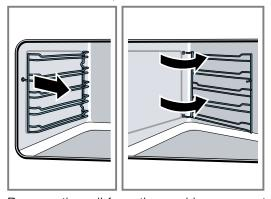
**3.** Remove the rail from the cooking compartment.
