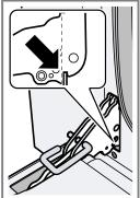
The notch below the hinges must engage into the frame of the appliance.
