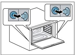
5. Screw the appliance tightly onto the unit.
