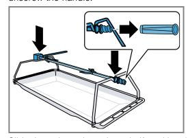
**3.** Slide the universal pan into shelf position 1 and place the rotary spit into the motor bracket.
