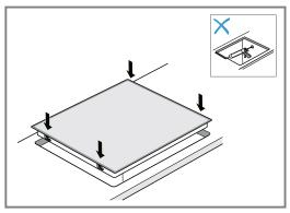
Seal the tile joints on tiled work surfaces with silicone rubber.
