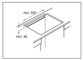
**3.** If the clearance from the back wall of the unit is less than 20 mm, create an opening on the underside.
