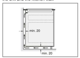
2. Ensure that an opening at the top of the rear of the unit is unobstructed.
