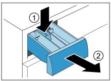
3. Pull out the insert upwards.
