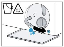
8. Firmly press on the sealing cap.
