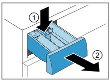
3. Pull out the insert upwards.
