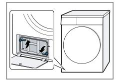
Pull out the heat exchanger cover by the handle.
