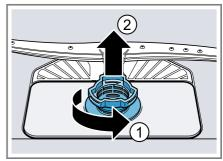
Pull down the micro filter to remove.
