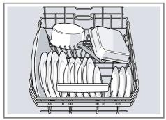
Large plates up to a diameter of 31 cm can be arranged in the bottom basket as shown.
