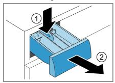
**3.** Pull out the insert upwards.
