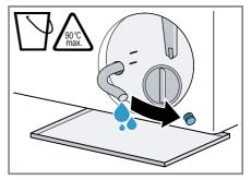
8. Firmly press on the sealing cap.
