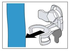
2. Unscrew ① and remove ② all the screws for the 4 transit bolts with a WAF 13 wrench.
