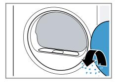
3. Remove the two-part fluff filter.
