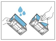
You can remove heavy soiling carefully with a soft brush. Ensure that you thoroughly dry off the filter. If the filter is damp, this may increase the drying time and affect the drying result. 4. Pull the fluff collector out horizontally.
