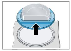
4. Turn the door ring by 180 1 and insert the door into the door ring 2
