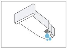
Check the condensation container filter  $\rightarrow$  Page 53 regularly and clean the filter if it is dirty. Make sure that you insert the con-
