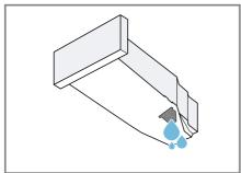
**5.** Remove the stopper on the underside.
