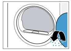
3. Remove the two-part fluff filter.
