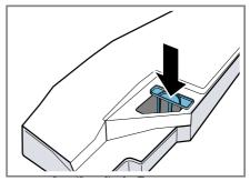
5. Insert the condensation container. → "Inserting the condensation container". Page 30
