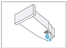
Check the condensation container filter → Page 33 regularly and clean the filter if it is dirty. Make sure that you insert the condensation container before operating the appliance.
