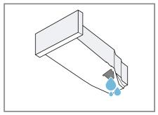
Check the condensation container filter → Page 48 regularly and clean the filter if it is dirty. Make sure that you insert the condensation container before operating the appliance.
