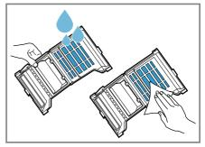
You can remove heavy soiling carefully with a soft brush. You must not damage or remove the fluff collector's seal. You can clean the fluff collector in the dishwasher.
