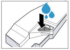
Hold the full condensation container level so that no liquid spills out. **3.** Insert the condensation container so that it locks into place.
