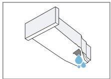
**5.** Remove the stopper on the underside.
