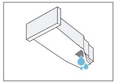
Check the condensation container filter  $\rightarrow$  Page 50 regularly and clean the filter if it is dirty. Make sure that you insert the condensation container before operating the appliance.
