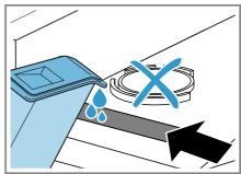
Check the water tank filter regularly and clean the filter if it is dirty. → "Cleaning the water tank filter", Page 49
