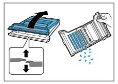
**6.** Clean the filter thoroughly under running water and then dry it off.
