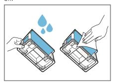
You can remove heavy soiling carefully with a soft brush. Ensure that you thoroughly dry off the filter. If the filter is damp, this may increase the drying time and affect the drying result.
