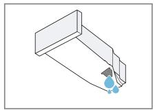
5. Remove the stopper on the underside.
