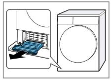
The fluff collector may contain condensation, which may drip out of it when you pull it out. **5.** Open the fluff collector and remove any fluff.
