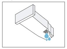
Check the condensation container filter → Page 50 regularly and clean the filter if it is dirty. Make sure that you insert the condensation container before operating the appliance.
