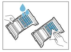
You can remove heavy soiling carefully with a soft brush. You must not damage or remove the fluff collector's seal. You can clean the fluff collector in the dishwasher.
