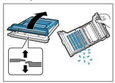
**6.** Clean the filter thoroughly under running water and then dry it off.
