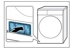
2. Close the lever for the heat exchanger.
