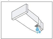
**6.** Insert the condensation container so that it locks into place.
