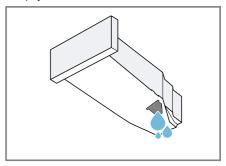
Check the condensation container filter → Page 42 regularly and clean the filter if it is dirty. Make sure that you insert the condensation container before operating the appliance.
