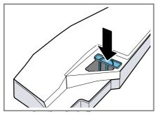
5. Insert the condensation container. → "Inserting the condensation container", Page 31 You can rectify minor faults on your appliance yourself. Read the troubleshooting information before contacting after-sales service. This will avoid unnecessary costs.
