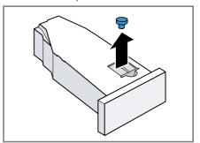
2. Insert the stopper on the underside.
