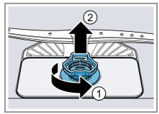
Pull down the micro filter to remove.
