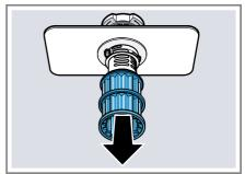
Press the locking catches ① together and lift the coarse filter out ②.
