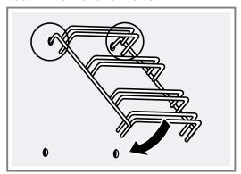
4. Hook both rails into the side walls of the oven.
