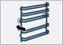
The rails fit both on the left and right sides. Shelf positions 1 and 2 are located at the bottom and shelf positions 3, 4 and 5 are located at the top.
