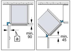
Observe the minimum dimensions in a corner installation in order to be able to open the cover of the appliance. The dimension a depends on the thickness of the furniture panel and the handle.
