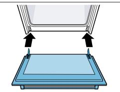
2. The notch on the hinge must engage on both sides.
