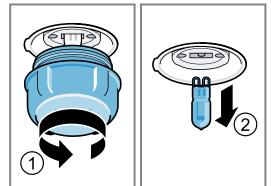
4. Insert the new halogen bulb and press it firmly into the socket.
