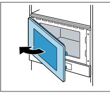
4. Screw the appliance to the unit on the opposite side to the hinges.
