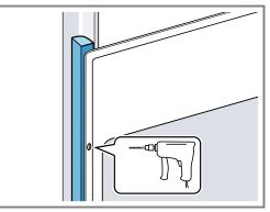
4. Secure the appliance using a suitable screw.
