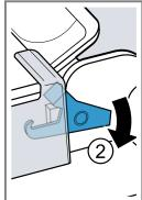
The locking levers are closed. The appliance door is secured and cannot be detached.
