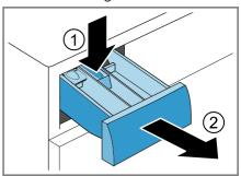
3. Pull out the insert upwards.
