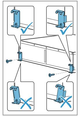
**6.** Slide the appliance into the fitted unit and check whether the tilt protection engages.
