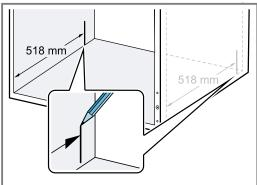
2. Screw the two brackets into the elongated hole behind the mark.
