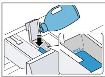
Do not exceed the marking for the maximum fill level when filling.
