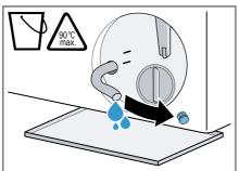
8. Firmly press on the sealing cap.
