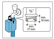
When connecting to a 21 mm = ½" tap, first fit the adapter with a sealing washer.
