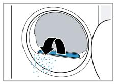
Ensure that no fluff falls into the air channel.
