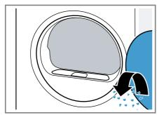
3. Remove the two-part fluff filter.
