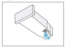
Check the condensation container filter → Page 41 regularly and clean the filter if it is dirty. Make sure that you insert the condensation container before operating the appliance.
