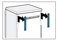
3. Undo and remove the screws in the horizontal transport strut using a T20 screwdriver.
