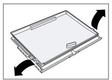
4. Lift the cover at the front 1 and pull it out at the rear 2.
