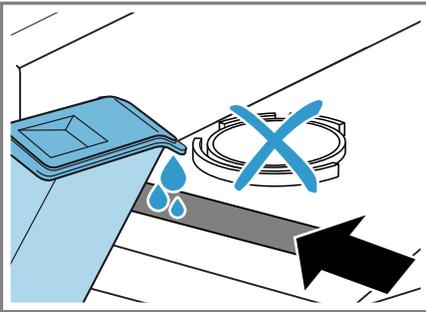
Check the water tank filter regularly and clean the filter if it is dirty.
