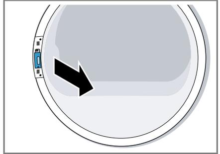
4. Assemble the door lock on the other side.
