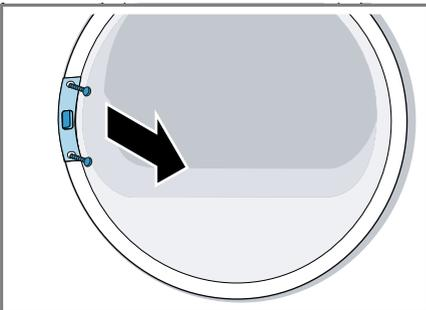
3. Disassemble the door lock.
