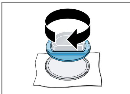
4. Place the door onto the door ring in the correct position.
