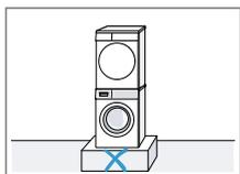
Only use the original connection set from the dryer manufacturer when setting up this appliance in a washer-dryer stack.
