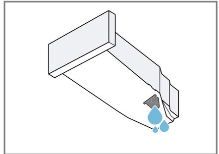
5. Remove the stopper on the under-side.
