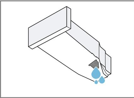
Check the condensation container filter → *Page 58* regularly and clean the filter if it is dirty. Make sure that you insert the condensation container before operating the appliance.
