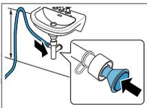
Secure the connection point with a (12-22 mm) hose clamp. Secure the water drain hose with a hose guide at a height of at least 80 cm and no more than 100 cm.
