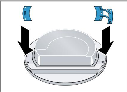
2. Disassemble and take off the door lock cover.
