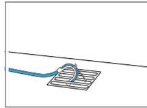
Push the water drain hose fully through the and secure it using fixing material. Secure the elbow to the gully.
