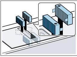
6. Insert the grease filter.
