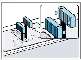
Insert the other odour filters or acoustics filters into the left and right of the appliance.
