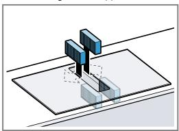
6. Insert the grease filter.
