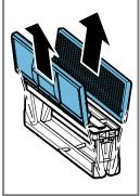
2. Place the grease filters loosely in the dishwasher and do not jam it in.
