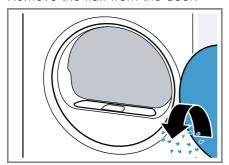
3. Remove the two-part fluff filter.
