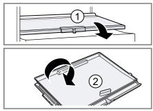
**3.** Press the fastenings for the lower cover outwards.
