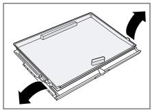
4. Lift the cover at the front ① and pull it out at the rear ②.
