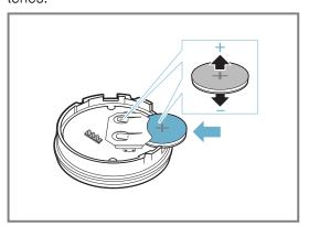
Note: Do not use any metal objects to remove the battery. Do not touch the battery connection points.
