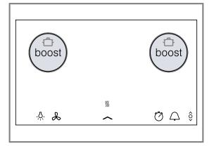
If the function is activated and you select a second cooking zone on the same side of the cooking surface, the appliance deactivates the function. The appliance automatically sets power level 9.0.
