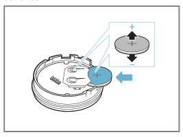
Note: Do not use any metal objects to remove the battery. Do not touch the battery connection points. 4. Close the cap on the cooking sensor. The indentations for the screws on the cap must be aligned with the indentations on the lower section of the housing. Use a screwdriver to tighten the screws and secure the silicone cover on the lower section of the cooking sensor housing.
