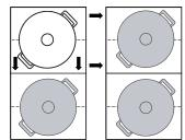
The cookware is detected. After a few seconds, the option to confirm the default settings for the new cooking zone appears on the display.
