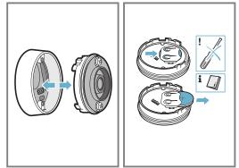
**3.** Insert a new battery, observing the instructions for the battery poles. Only use premium-quality CR2032 batteries.
