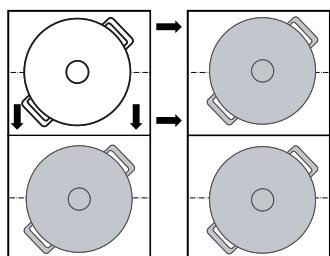
The cookware is detected. After a few seconds, the option to confirm the default settings for the new cooking zone appears on the display.
