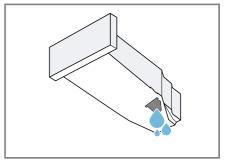
Check the condensation container filter  $\rightarrow$  Page 42 regularly and clean the filter if it is dirty. Make sure that you insert the condensation container before operating the appliance.
