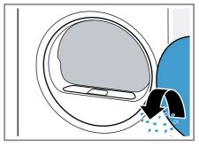
**3.** Remove the two-part fluff filter.
