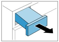
**6.** Add approx. 1 <sup>1</sup>/<sub>2</sub> litres of hot tap water into the condensation container.
