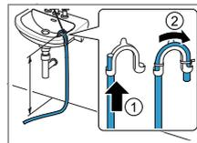
Push the water drain hose fully through the elbow and secure it using fixing material. Secure the elbow at a height of no more than 100 cm.
