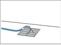
bow and secure it using fixing material. Secure the elbow to the gully.
