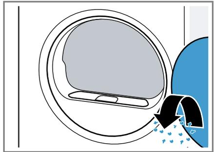
3. Remove the two-part fluff filter.
