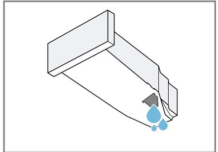
Check the condensation container filter → *Page 37* regularly and clean the filter if it is dirty. Make sure that you insert the condensation container before operating the appliance.
