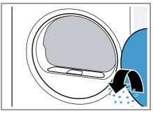
**3.** Remove the two-part fluff filter.
