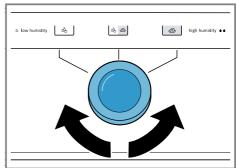
The air humidity in the fruit and vegetable container can be set according to the type and amount of food to be stored by turning the humidity control:
