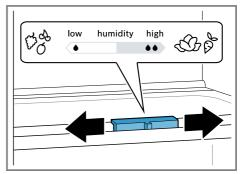
The air humidity in the fruit and vegetable container can be set according to the type and amount of food to be stored by moving the humidity controller:
