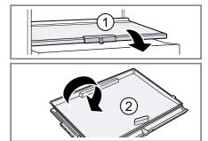
**3.** Press the fastenings for the lower cover outwards.
