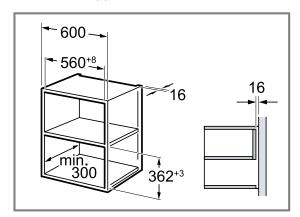
Do not fit the appliance too high up; it must be possible for accessories to be removed easily. Remove the feet.
