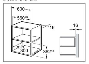
Do not fit the appliance too high up; it must be possible for accessories to be removed easily. Remove the feet.
