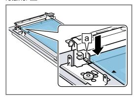
4. Slide in a second intermediate pane. When doing so, ensure that the number on the intermediate pane is at the bottom right 1.
