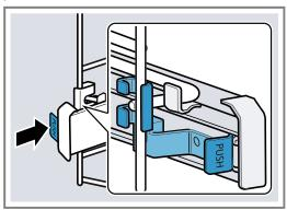
2. Keep the PUSH tab pushed back ① and swing the rail outwards 2.
