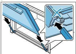
2. Using both hands, press down on the left and right of the door cover from above to check whether the appliance has been pushed in as far as it will go.
