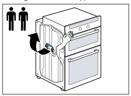
3. Place the appliance in the unit and fold the carry handles down.
