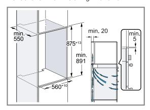
To ventilate the appliance, there must be a gap of 20 mm between all intermediate floors and the wall.
