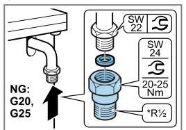
3. Secure the connecting piece using a 24 mm spanner. Use a 24 mm spanner to place the threaded fitting of the gas pipe or safety gas hose on the connecting piece and tighten it firmly.
