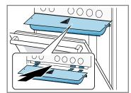
**Note:** There are three notches below the control panel. Insert the three lugs on the protecting plate into the three notches.
