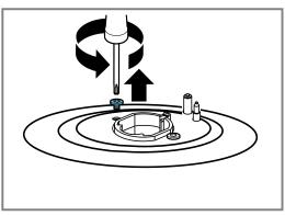
**4.** Remove the two screws (T20) at the front right and left of the hob panel. Do not remove the plastic parts that are located below these.
