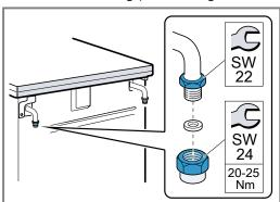
3. After changing the connection side, carry out a leak test. You can find additional information about this in the section entitled "Leak and function test" → Page 35.
