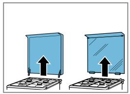
2. Remove the pan support grids or the pan support racks and the burner parts.
