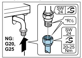
**4.** Open the gas connection shut-off. Carry out a leak test → Page 35.
