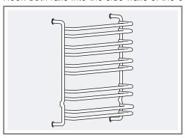
If the rails are fitted correctly, the distance between the two upper shelf positions is greater.
