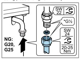
5. Open the gas connection shut-off. Carry out a leak test → Page 35.
