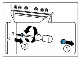
Remove the two screws (M4) that are uncovered when you remove the control knobs (T15).
