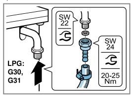
Fit the safety gas hose and use a pipe union or cable clamp to tighten it securely.
