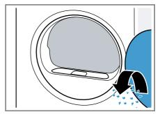
3. Remove the two-part fluff filter.
