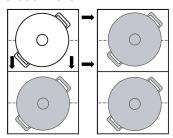
The cookware is detected and the previously selected power level and  $\xi$  flash alternately on the display for the new cooking zone.
